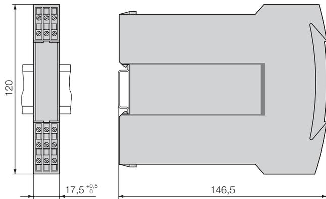
Fig. 4. SINEAX SV 824 in housing S17 clipped onto a top-hat rail (35x15 mm or 35x7.5 mm, acc. to EN 50 022)
