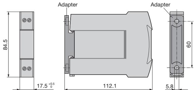
Fig. 11. SINEAX TI 807-5.... (housing **N17**) with adapter for directly wall mounting.
