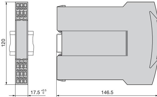
Fig. 12. SINEAX TI 807-1.... (housing **S17**) clipped onto a top-hat rail (35 x 7.5 or 35 x 15 mm, acc. to EN 50 022).
