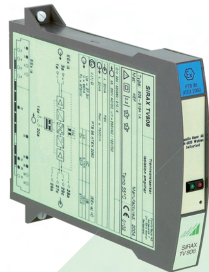
Fig. 1. Steck-Modul SIRAX TV 808-61 for plugging onto backplane BP 902.
