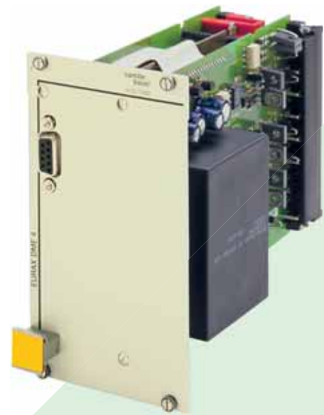
Fig. 1. EURAX DME 424 as plug-in module for 19" rack-mounted case, front plate width 14 TE.
