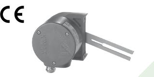
Fig. 1. Position feedback transmitter KINAX SR 719 showing the operating lever in the lower zero position, corresponding output current 4 mA.
