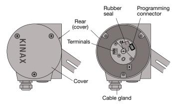
Fig. 8. KINAX SR 719 with screw terminals and cable gland.
