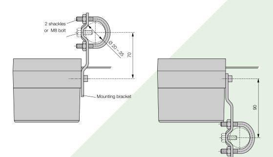
Fig. 11. KINAX SR 719 with fitting recommended by NAMUR.
