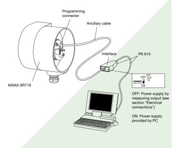
Fig. 7. Example of the set-up for programming a KINAX SR 719 without the power supply. For this case the switch on the interface must be set to «ON».
