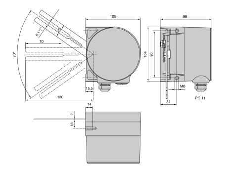
Fig. 10. Position of the KINAX SR 719 operating lever in the upper zero position, corresponding output current 4 mA.
